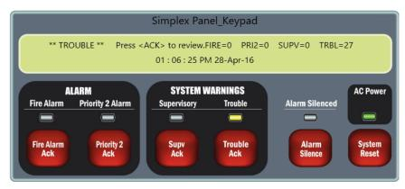
The messages displayed in the text field indicate the number of points that have Alarms and System Warnings. The LED lights on the Virtual Keypad are color coded to indicate the status of the fire panel. The table below lists the alarm definitions for each color:
