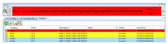
Selecting an individual event from the expanded view allows sending of commands to the device.
